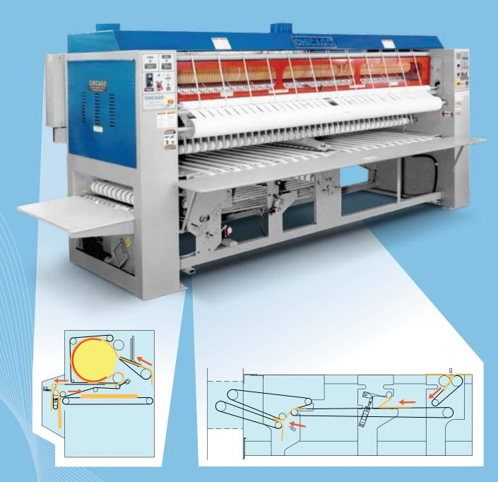
Series of precise air-blasts folds with pinpoint accuracy resulting in neatly finished items.
