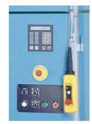
The controls are composed of two (2) basic sections: the drying controls and the load/unload controls.
